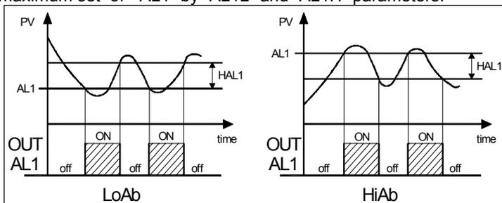
**LodE** = DEVIATION LOW ALARM: The alarm is activated when the process value goes below the value [SP1 + AL1] and will be deactivated when it goes above the value [SP1 + AL1 + HAL1].
