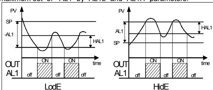
**LHAb** = ABSOLUTE BAND ALARM: The alarm is activated when the process value goes under the alarm threshold set on parameter "AL1L" or goes higher than the alarm threshold set on parameter "AL1H" and will be deactivated when it goes below the value [AL1H - HAL1] or when it goes above the value [AL1L + HAL1].
