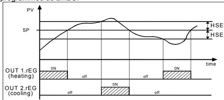
If 2.rEG output is used to control compressor is possible to use the "Compressor Protection" function that has the meaning to avoid compressor "short cycles".
