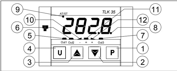
**1 - Key P** : This is used to access the programming parameters and to confirm selection.
