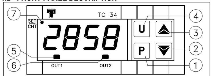
1 - Key P : Used for the set point setting and to program the functioning parameters
