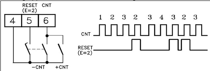
With this UP/DOWN counting applications the counting cannot assume negative values and therefore reached the value 0 (counting UP) or the set value (counting DOWN) others pulses can't be acquired.
