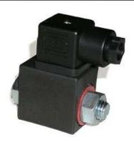
This coil is usually installed on dyeing machine pipe, in order to detect the passage fo a magnet put inside the fabric. It is connected to a seam detector that work as signal amplifier. The GS coil has an additional iron bolt and nuts to enhance magnet detection.
